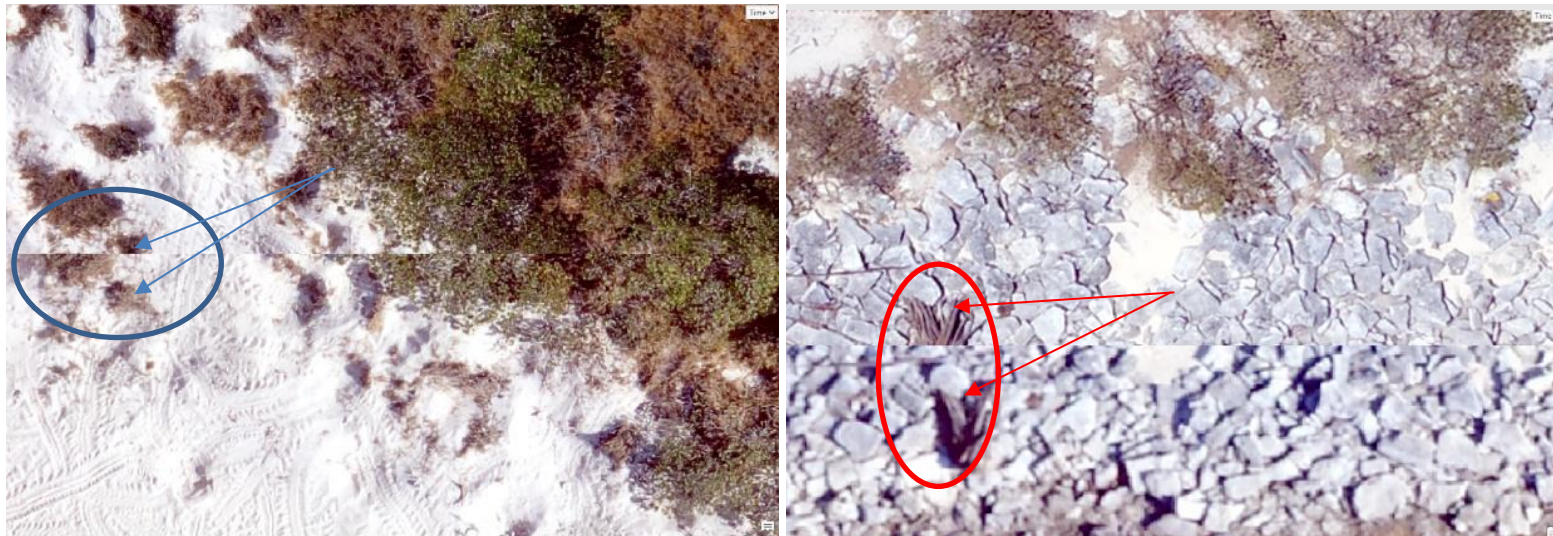
Fig. 4.1 Examples of the variation in spatial accuracy between orthomosaics. Arrows point to identical features in two orthomosaics of the same location.
