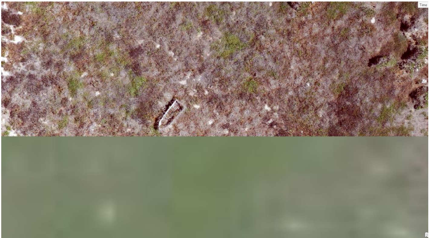
Fig. 4.2 The upper section of the image shows the resolution and detail obtained from the drone on South West Islet and the abandoned aluminium Hercules boat. The lower section shows the typical resolution from global satellite data sets.
