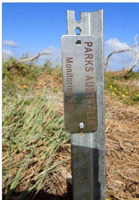
Figure 3. Permanent sites are marked using galvanized star pickets labelled with Parks Australia stainless steel identification tags. Photo: Joy Brushe
