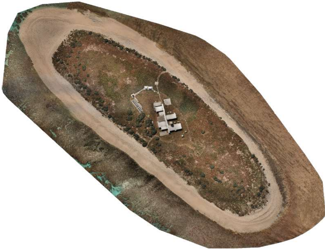
Figure 62. South Islet orthomosaic preview (Pix4DEngineSDK version 5.0.45), showing the entire island (coral sand beaches, vegetation and station infrastructure), as well as a portion of the exposed reef (low tide). Credit: Dan Wilkins ©, Parks Australia.
