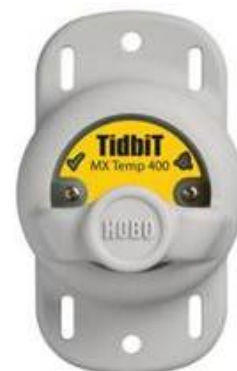
Figure 19. HOBO MX2203 TidbiT Bluetooth data logger.
