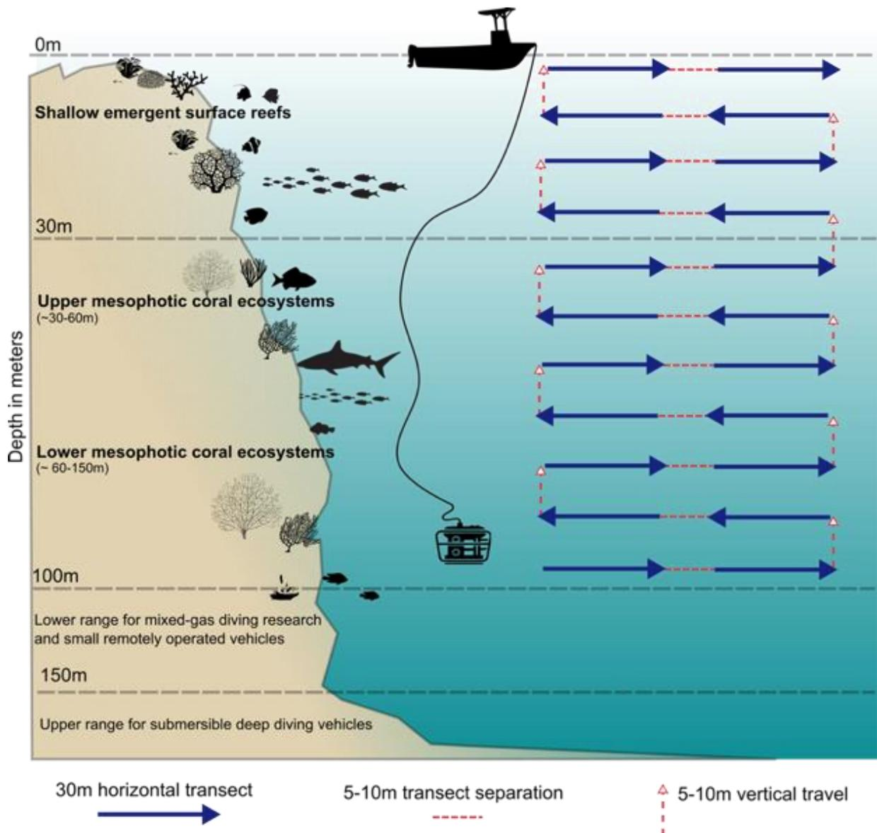
**Figure 3.6** Remotely Operated Vehicle (ROV) transect survey methodology used to survey fish and benthic communities in the Coral Sea Marine Park. All ROV surveys were conducted at depths between 10 – 80m using the BlueRobotics BlueRov2.
