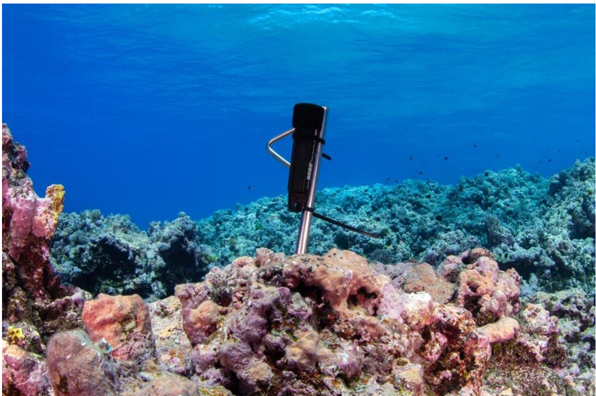
Figure 3.4 Photographs of crustose coralline algae (CCA) devices and temperature loggers deployed in Feb-Mar 2023 and Feb-Mar 2024. Top: CCA devices deployed on the reef slope of Osprey Reef. Bottom: Hobo temperature logger deployed on the reef crest at Willis Islets. Image credits: Victor Huertas.
