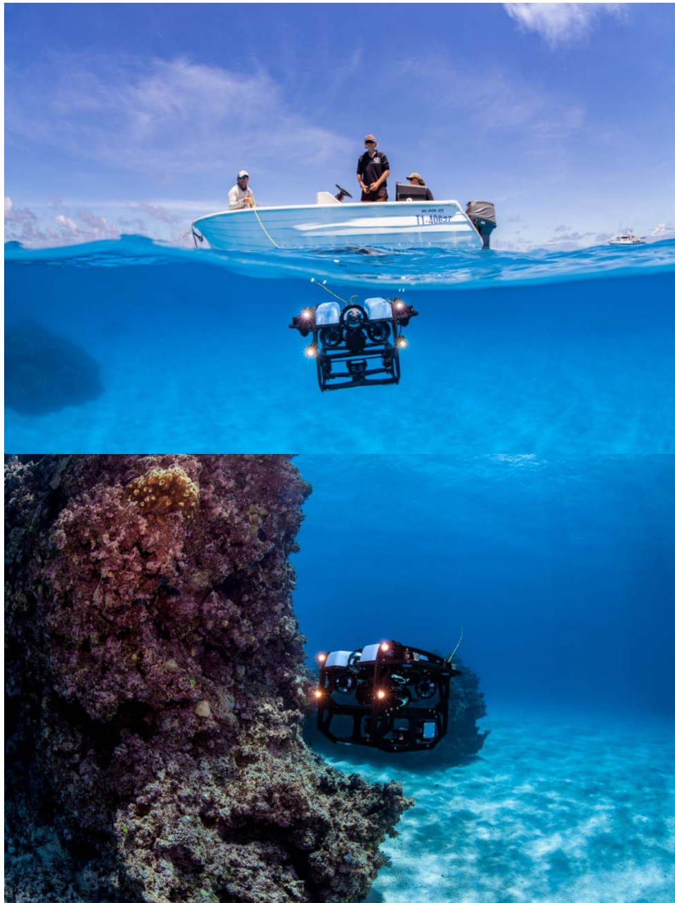
Figure 3.2 – Photographs showing the operation of the Remotely Operated Vehicle (ROV) from a tender to the MV Iron Joy in the Coral Sea Marine Park. Top: The ROV being deployed from the tender with the operator (Gemma Galbraith, standing) piloting the ROV, while an assistant manages the tether (Ben Cresswell). Bottom: The ROV navigating around a shallow bommie. Image credits: Victor Huertas
