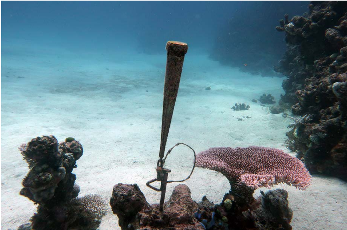
Figure 4.4 A Marriot HS (high sampling rate) drag and tilt current meter deployed at approximately 10m on a reef in the southern Coral Sea Marine Park. This current meter was deployed in February 2019 and the photo taken immediately prior to retrieval in February 2020. Image credit: Martin Russell
