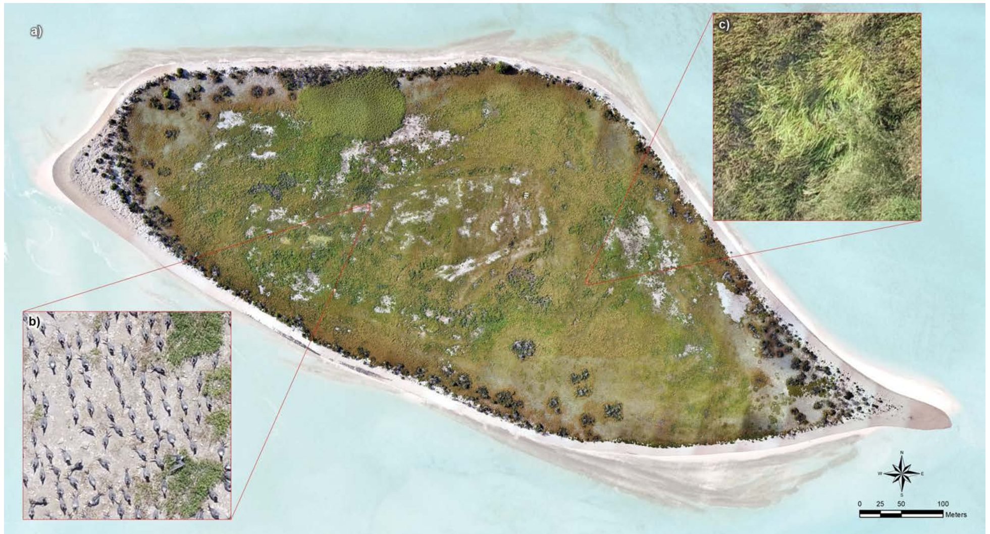
Figure 5. Orthomosaic image of West Island at Ashmore Reef in May 2019 (a). RPAS missions flown at 30 m altitude were of sufficient resolution to identify individual birds to species (b) and spot introduced plant populations for subsequent ground truthing (c). Insets depict (b) nesting crested terns ( Thalasseus bergii ) and (c) burr grass ( Cenchrus brownii ). Background imagery dates from October 2016, which explains the slight misalignment of the island coastline due to erosion and accretion over time.
