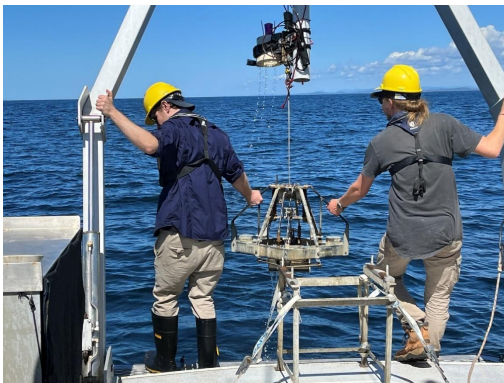
Figure 2.6 Smith-MacIntyre grab (near stand) with USBL and GoPro (top of picture) armed and ready for deployment, RV Bombora; credit Tom Doyle.
